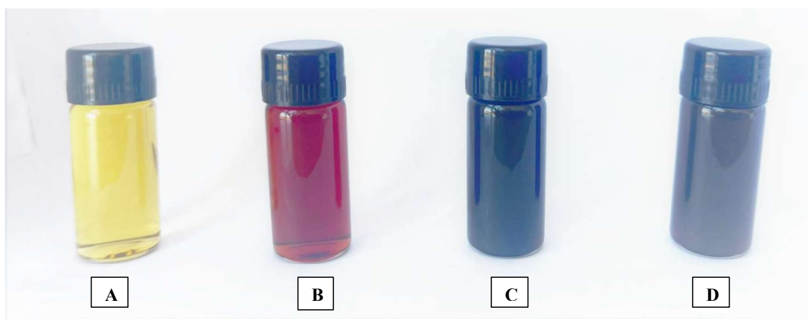
Figure 01: Colloidal silver dispersions. A: Silver nanoparticles. B: silver nanoparticles with glycolic acid (1:1); C: silver nanoparticles with glycolic acid (1:5) D: silver nanoparticles with glycolic acid (1:10)
